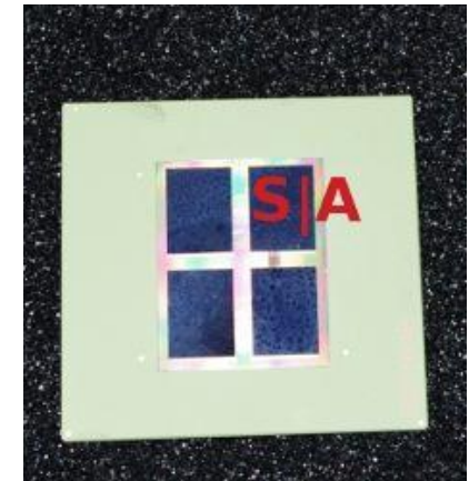
IBM Power 7+: four 32nm CMOS multi-core CPU dies are placed side by side on a silicon Interposer. (Courtesy of SemiAccurate.com)
